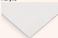
Acrylic is resistant to long-term sunlight exposure and weathering. It has excellent optical properties and a much higher impact resistance than glass. Acrylic has low water absorption, good electrical resistivity, and fair tensile strength. It can be routed, drilled, flame polished, and bent into many shapes, perfect for applications including glazing, windows, signage, POP, screens, transparent barriers, signage, and lighting.
