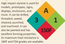
• Outstanding thermoforming characteristics
