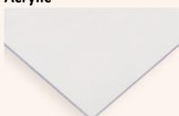
Acrylic is resistant to long-term sunlight exposure and weathering. It has excellent optical properties and a much higher impact resistance than glass. Acrylic has low water absorption, good electrical resistivity, and fair tensile strength. It can be routed, drilled, flame polished, and bent into many shapes, perfect for applications including glazing, windows, signage, POP, screens, transparent barriers, signage, and lighting.
