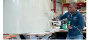
FUSION 3C during the welding of a fillet weld.
