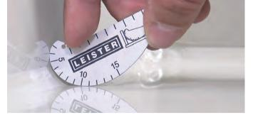
Check the weld seam dimension easily.
