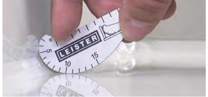
Check the weld seam dimension easily.
